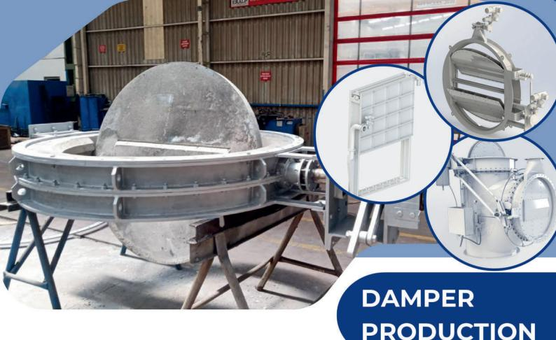
As Fortek Industrial, we manufacture a wide range of dampers for power plants and industrial plants to control or shut off the gas flow in a fully sealed manner. We advise on selecting the right damper and actuator type and ensure that the most efficient design choices are made from the outset of the project. Careful planning in advance ensures that the end customer receives the ideal and best working damper systems for each application.
