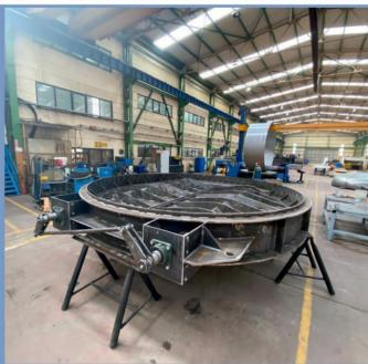
FORTEK 2-WAY DAMPERS PROVIDE A SIMPLE AND COST-EFFECTIVE METHOD OF CONTROL AND ISOLATION. A VARIETY OF SEALING SYSTEMS, INCLUDING SPECIAL ALLOY SPRINGS AND AIR FANS, CAN BE USED TO PROVIDE THE CORRECT SEALING EFFICIENCY REQUIRED FOR YOUR APPLICATION.
