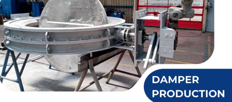
Fortek Industrial manufactures a wide range of dampers for power plants and industrial plants to control or shut off the gas flow in a fully sealed manner. We advise on selecting the right damper and actuator type and ensure that the most efficient design choices are made from the outset of the project. Careful planning in advance ensures that the end customer receives the ideal and best working damper systems for each application.
